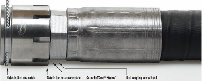
Holes in iLok nut match grooves in female end when fully tightened, allowing passage of a cable to prevent nut from backing off.
